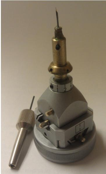
Figure 3, Goniometer head and adjustment screw
