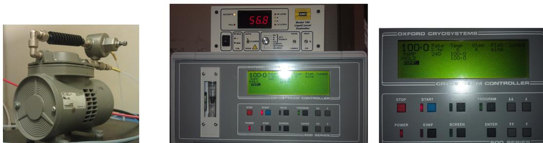
**Figure 1, The circulation pump and the two external controllers for the Oxford Cryosystems variable temperature unit.**
